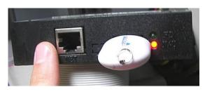
2. Once the USB stick is plugged in, follow the normal path or operator steps to access a "Floppy Disk" or to write to a "Floppy Disk" on the machine. Both the **RED** <u>AND</u> **GREEN** light should come on throughout the process of reading or writing on the USB stick.
